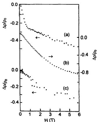
Fig. 3.  $\Delta\rho/\rho_0$  as a function of applied magnetic field at 4.2 K for samples (a) E, (b) Y and (c) B.
