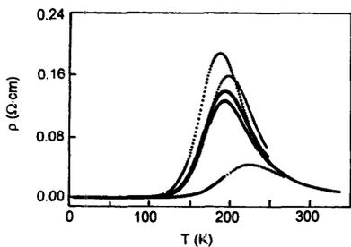
Fig. 2. Resistivity as a function of temperature for different field values for the sample Y. Curves with decreasing peak height correspond to applied fields of 0, 0.5, 1.0, 2.0, and 5.0 Tesla, respectively.
