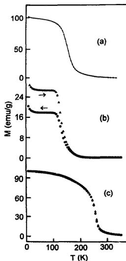
Fig. 4. Temperature dependence of magnetization in a field of 1.0 Tesla for samples (a) E, (b) Y and (c) B.
