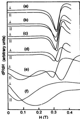
Fig. 6. Ferromagnetic resonance (FMR) spectra recorded in the parallel and perpendicular geometries for sample E at different temperatures; (a) 298 K, (b) 273 K, (c) 223 K, (d) 173 K, (e) 148 K and (f) 123 K.
