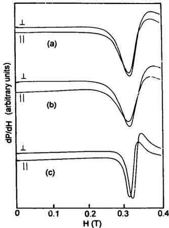
Fig. 5. Ferromagnetic resonance (FMR) spectra recorded in the parallel and perpendicular geometries at 298 K for samples (a) E, (b) Y and (c) B.
