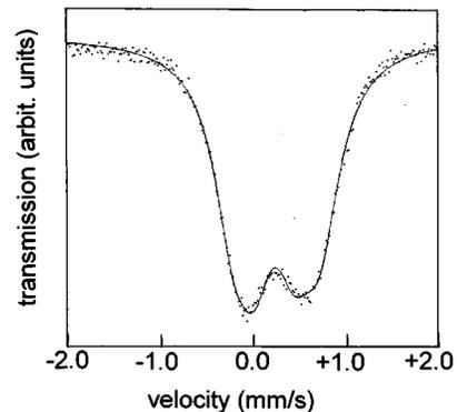
FIG. 3. Room temperature  $^{57}\text{Fe}$  Mössbauer effect spectrum of icosahedral  $\text{Al}_{50}\text{Pd}_{10}\text{Mn}_{20}\text{Fe}_5\text{B}_{15}$ . The solid line is a fit to two symmetric doublets.
