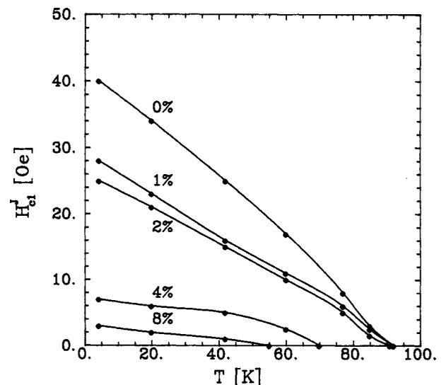
Fig. 4.  $H_{c1}^I$  of  $\text{YBa}_2(\text{Cu}_{1-x}\text{Fe}_x)_3\text{O}_{7-\delta}$  as a function of temperature for  $0 \leq x \leq 0.08$ .
