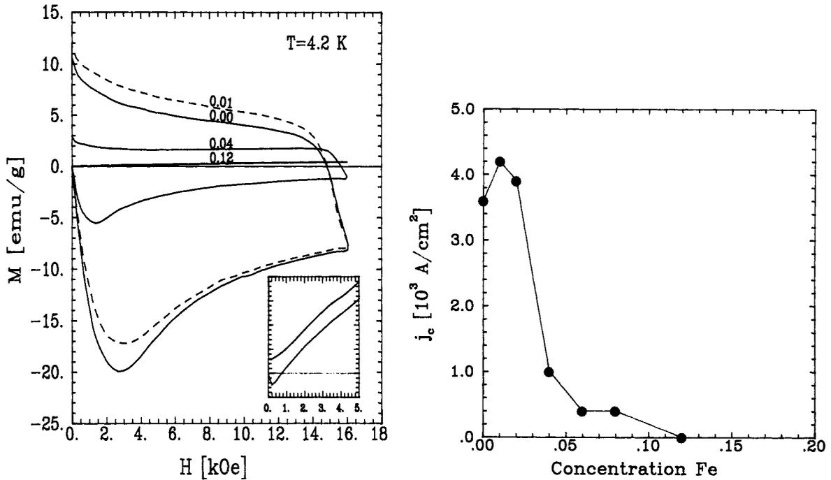
Fig. 3. (a) Hysteresis loops of  $\text{YBa}_2(\text{Cu}_{1-x}\text{Fe}_x)_3\text{O}_{7-\delta}$  at  $T = 4.2$  K, for  $x = 0, 0.01, 0.04$  and  $0.12$ , and (b) intragrain critical current density,  $j_c^G$ , as a function of  $x$ .
