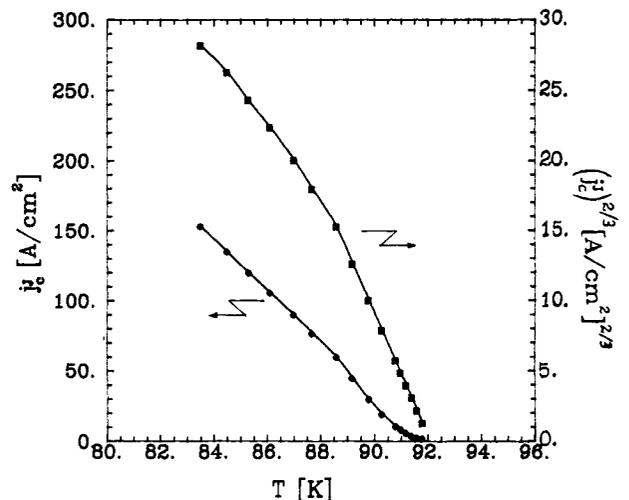
Fig. 7. Temperature dependence of  $j_c^I$  determined from  $\chi''$  peaks (left-hand scale) and plot of  $(j_c^I)^{2/3}$  (right-hand scale).
