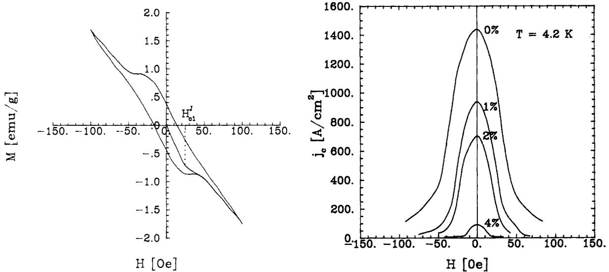
Fig. 5. (a) A typical low field hysteresis loop and (b) intergranular critical current density,  $j_c^I$ , of  $\text{YBa}_2(\text{Cu}_{1-x}\text{Fe}_x)_3\text{O}_{7-\delta}$  as a function of magnetic field for  $0 \leq x \leq 0.04$ .
