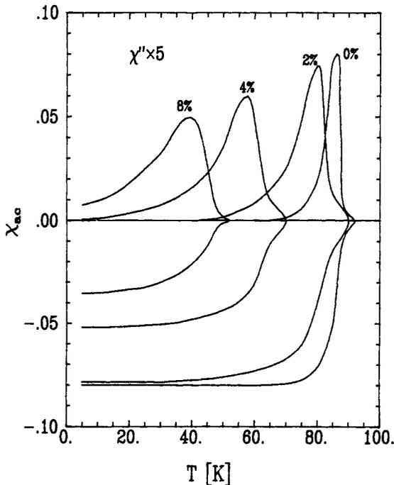
Fig. 6. Temperature dependence of the real and imaginary parts of complex susceptibility of  $\text{YBa}_2(\text{Cu}_{1-x}\text{Fe}_x)_3\text{O}_{7-\delta}$  for  $x = 0, 0.02, 0.04$  and  $0.08$ .
